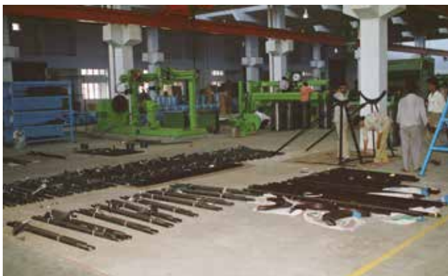
Stands for Solar Water Heaters being assembled at our fabrication unit.
