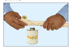
Without delay, while the solvent cement is still wet, assemble the pipe and fitting, and while doing so twist a ¼ turn as the pipe is being inserted (if possible), Once the pipe end has reached the fitting socket end, stop the insertion and rotation. Continuation of rotating further could break any fusion that is starting to occur.
